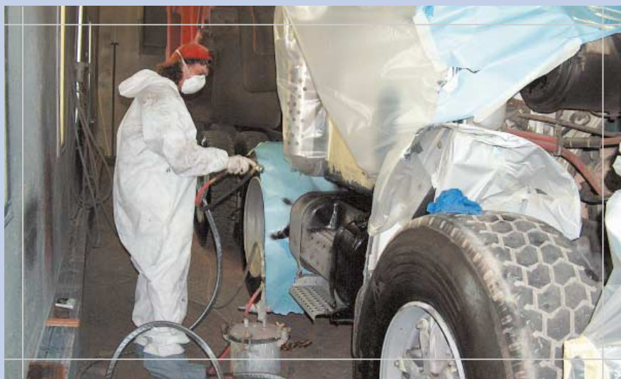
Photo: Darren Greer Sandblasting
